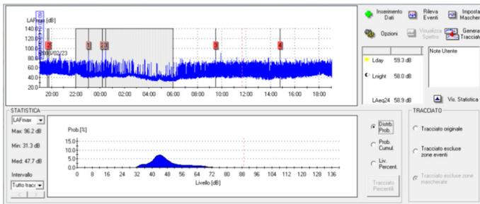
**Daily charts and events table:** daily processing allows to detect events on threshold conditions and to divide them over reference periods in a tabular format. Events detection function allows to search for impulses in the time profiles. Statistic is available both in graphic and numerical format as probability distribution, cumulative distribution and percentile levels.
