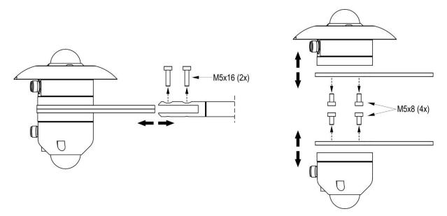
Fig. 6.1: disassembly of the pyranometers holder
