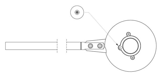
Fig. 4.1: position of bubble level
