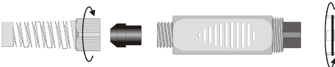
Open the two module shells: the printed circuit to which the probe must be connected is housed inside. On the left there are the 1...4 points on which the sensor wires must be welded. The JP1...JP4 jumpers are in the center of the board. For the 4-wire Pt100 sensor the jumpers must be left open.
