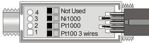
Before welding, pass the probe cable through the fairlead and gasket. Weld the wires as shown in the table:
