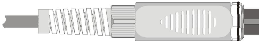
Make sure the cable is not twisted while you are screwing the fairlead. Now the probe is ready.
