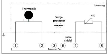
Scheme of principle LPPIRG01 (version with mV output)
