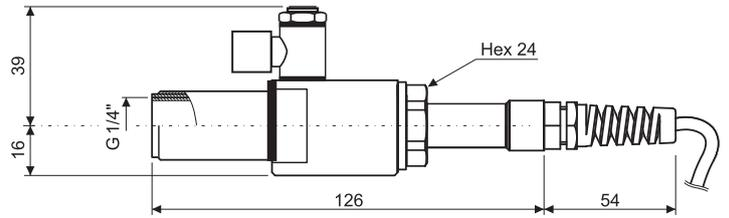
Dimensions (mm) of the probe with measuring chamber and quick coupling (only HP480):
