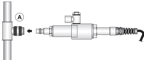
To connect with quick coupling, you can use one of the standard 1/4" couplings provided. Other couplings than those supplied can be used, provided that they have a G 1/4" thread on the side that fits into the probe.
