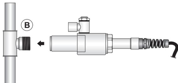
For the connection by threaded coupling, the connection must have an external G 1/4" thread on the side which will be placed in the probe. The connection must be airtight. When installing or removing the probe, it is necessary to depressurize the system.
