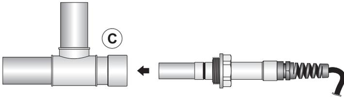
For direct connection of the probe, use a fitting with internal G 1/2" thread on the side which will be placed in the probe. The connection must be airtight. When installing or removing the model HP480, it is necessary to depressurize the system. Ensure that the probe does not obstruct the normal flow of air through the distribution line.
