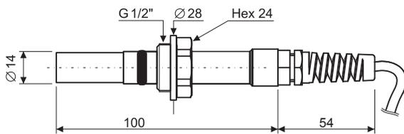
Dimensions (mm) of the probe with measuring chamber, without quick coupling (only HP480):
