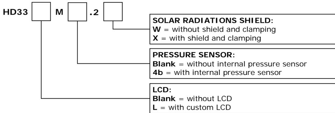
**HD33M-MB.2** GSM/GPRS data logger. RS485 MODBUS-RTU input and contact input for rain gauge. Stores measurements in the internal memory. Transmits the acquired data via FTP, via e-mail or to an HTTP server (Cloud). **Optional** LCD Display. Alarm functions. Power supply: 7...30 Vdc. It includes **HD35AP-S** software downloadable from Delta OHM web site.
