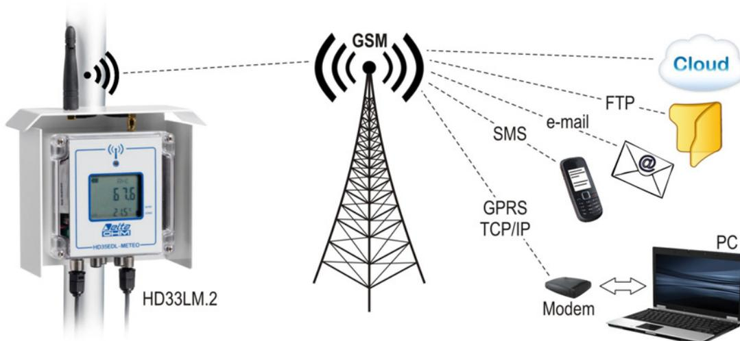
The data logger GSM functions can be remotely controlled by sending SMS messages.
