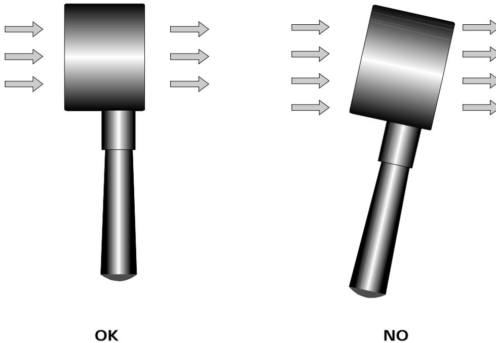
The probe is correctly positioned in relation to the air-flow when the value measured is the maximum possible.
