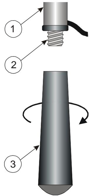
To mount the telescopic rod on the probes, unscrew the handle (3) holding the probe body still in the point (1). Screw the rod end on the screw (2). The handle (3) is screwed on the telescopic rod.
