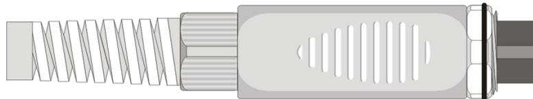
The instructions to connect the Platinum or Nickel probe to the module are provided below. The module is supplied complete with fairlead and gasket for 5 mm maximum diameter cables. Do the following to open the module and connect a probe:
