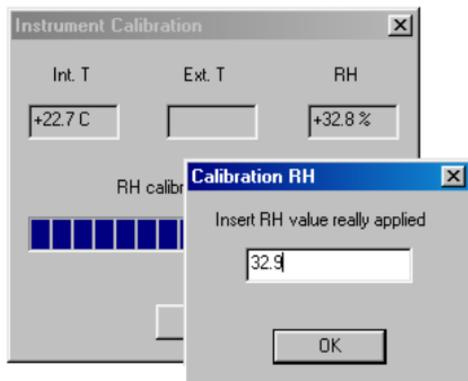
20. Take out the probe from the container with the 33%RH solution, then close it with its lid.
