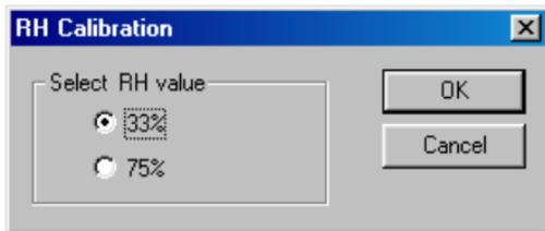
16. Take out the probe from the container with the 75%RH solution and close it with its lid, open the container with the 33%RH saturated solution. Check that inside the measuring chamber there are drops of solution: if any, blot them with paper.
