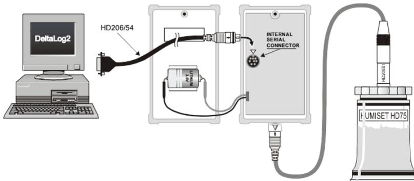
In all other cases, you just have to disconnect the external temperature or temperature/humidity probe, if any, and replace it with the serial cable supplied with DeltaLog2 program, as shown in the figure below.
