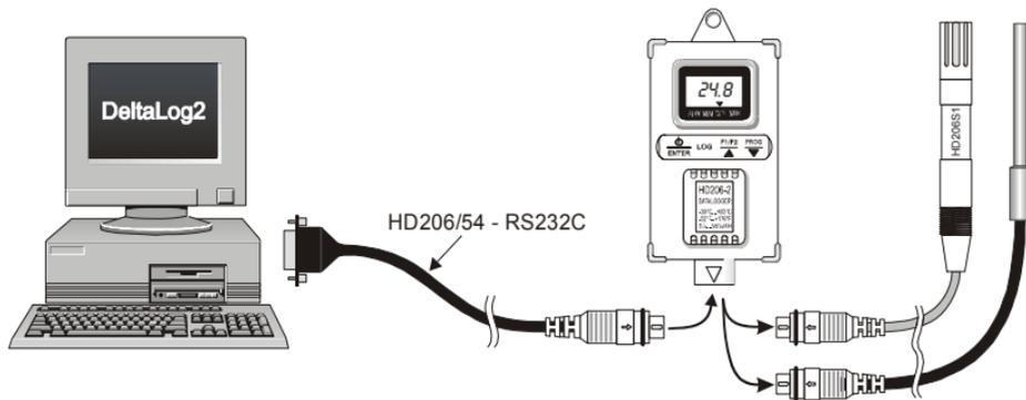
DeltaLog2 program allows to manage from your own PC all the minidatalogger functions in an easy and intuitive way: you can set logging start and stop times, alarm set-points, dump data and view them either in table or graphic format, display and save on file the measurements acquired from the instrument in real time, print data and export them in Excel<sup>®</sup> format, read the remaining battery charge... A password protects the instrument setup settings and prevents non-authorized changes.
