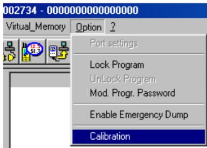
7. Enter **CAL** password (capital letters) and confirm. Select RH and confirm with OK. In the next window, select the first calibration point at 75%RH and press OK. The following window will appear. **Warning: do not confirm immediately!**
