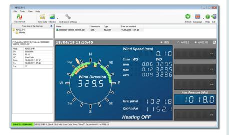
The PC software HD52.3D-S allows configuring the instrument, viewing the real time measurements both graphically and numerically, managing graphical presentation, printing and export in Excel® format of the data acquired with the Monitor function.
