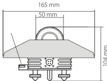
LPPYRA10 is also available in the version with shadow-ring (LPPYRA13). This measures the diffuse solar radiation eliminating the contribution of direct irradiance.
