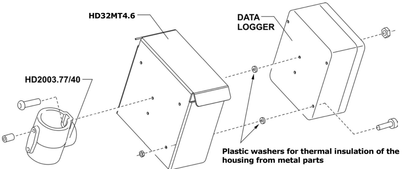
For outdoor installations, use the optional protection shield against solar radiations.
