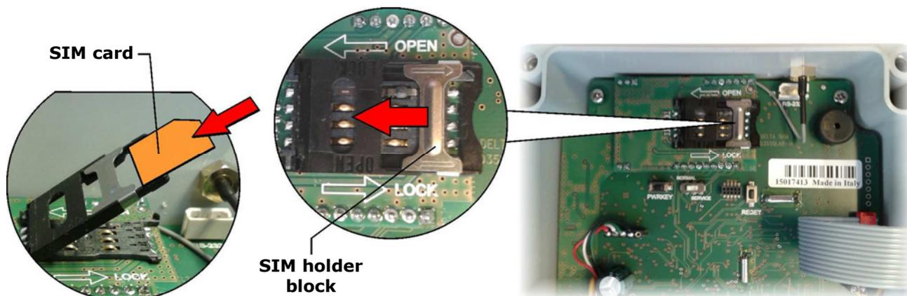
4. Insert the SIM card into its tray so as the SIM card contacts face down and correspond to the contacts on the electronic board. The SIM has to be inserted between the metal block and the plastic part.
