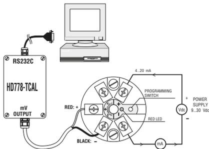
Instead of the thermocouple calibrator, you can use the Delta OHM HD778-TCAL: this instrument has to be connected to a serial port of the PC and, by means of a proper software, automates all the steps described below for programming the operating range.
