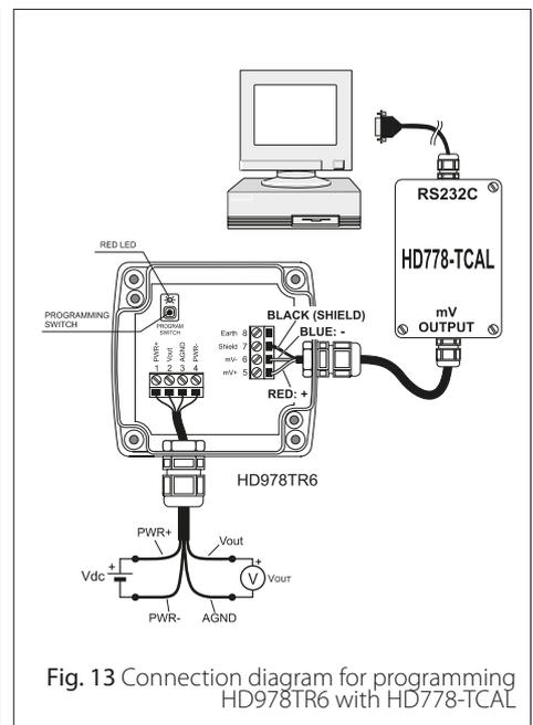
Fig. 13 Connection diagram for programming HD978TR6 with HD778-TCAL
