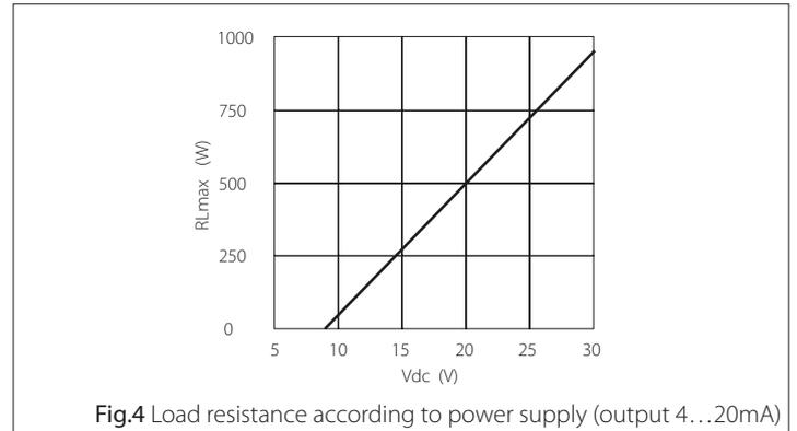
Fig.4 Load resistance according to power supply (output 4...20mA)
