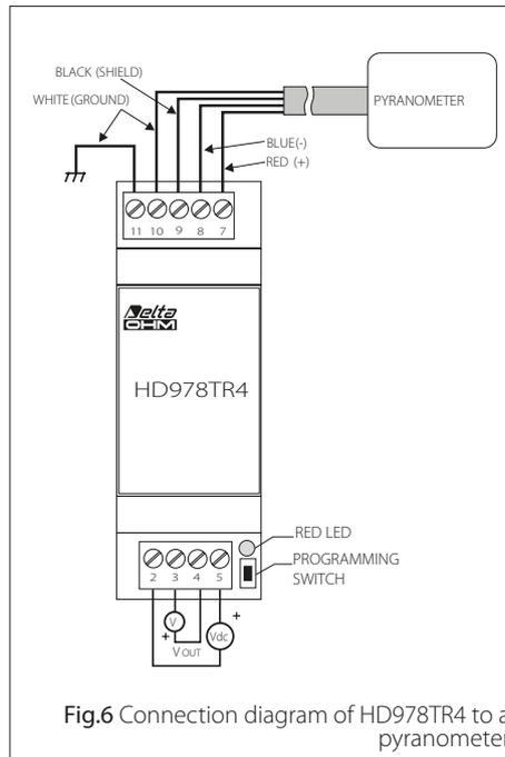
Fig.6 Connection diagram of HD978TR4 to a pyranometer
