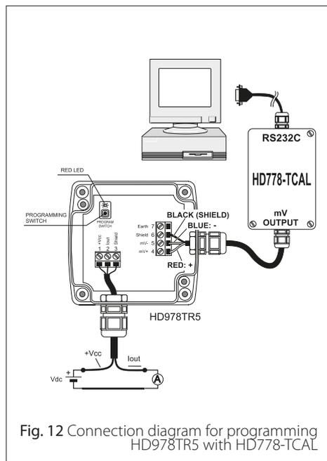
Fig. 12 Connection diagram for programming HD978TR5 with HD778-TCAL
