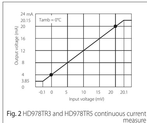
Fig. 2 HD978TR3 and HD978TR5 continuous current measure
