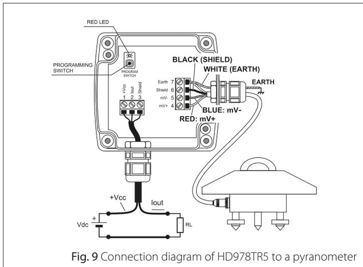
Fig. 9 Connection diagram of HD978TR5 to a pyranometer
