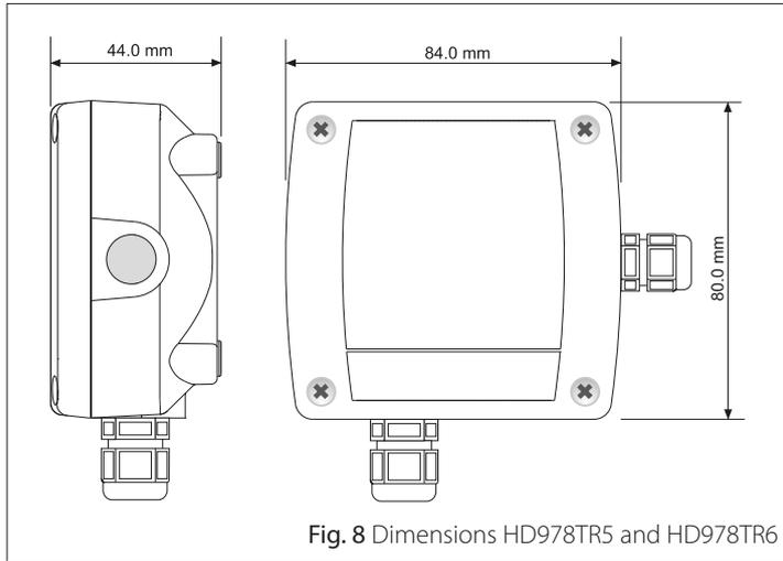
Fig. 8 Dimensions HD978TR5 and HD978TR6
