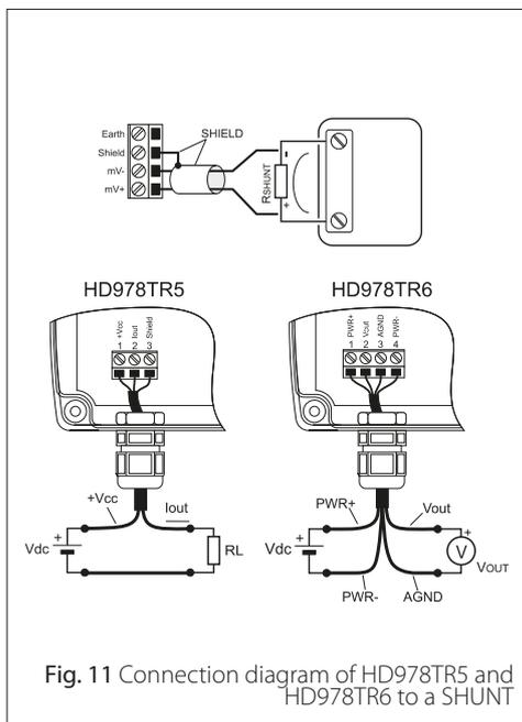
Fig. 11 Connection diagram of HD978TR5 and HD978TR6 to a SHUNT
