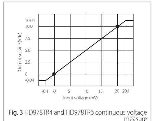
Fig. 3 HD978TR4 and HD978TR6 continuous voltage measure
