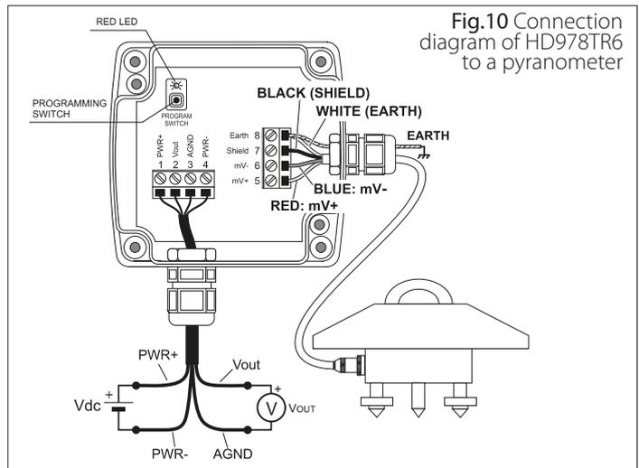
Fig. 10 Connection diagram of HD978TR6 to a pyranometer
