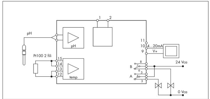
Fig.2 Passive transmitter.
